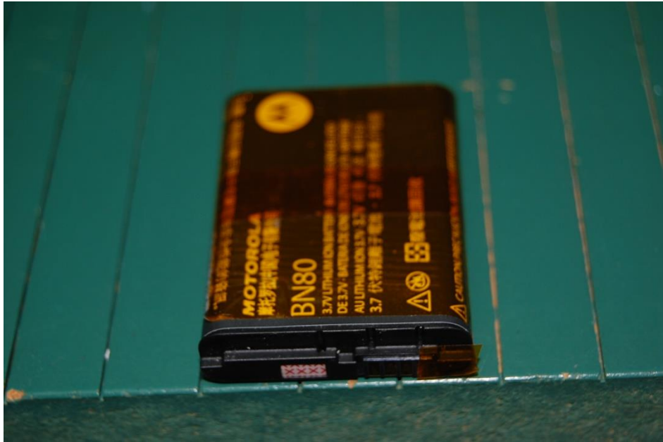
Figure 47 Kapton tape on body of battery
