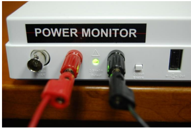
Figure 12 Vout LED indicator
