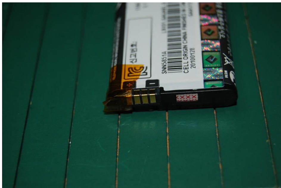
Figure 46 Kapton Tape on Terminals
