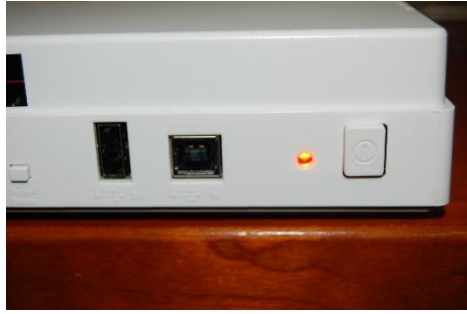
Figure 13 Amber LED indicator for over-current
