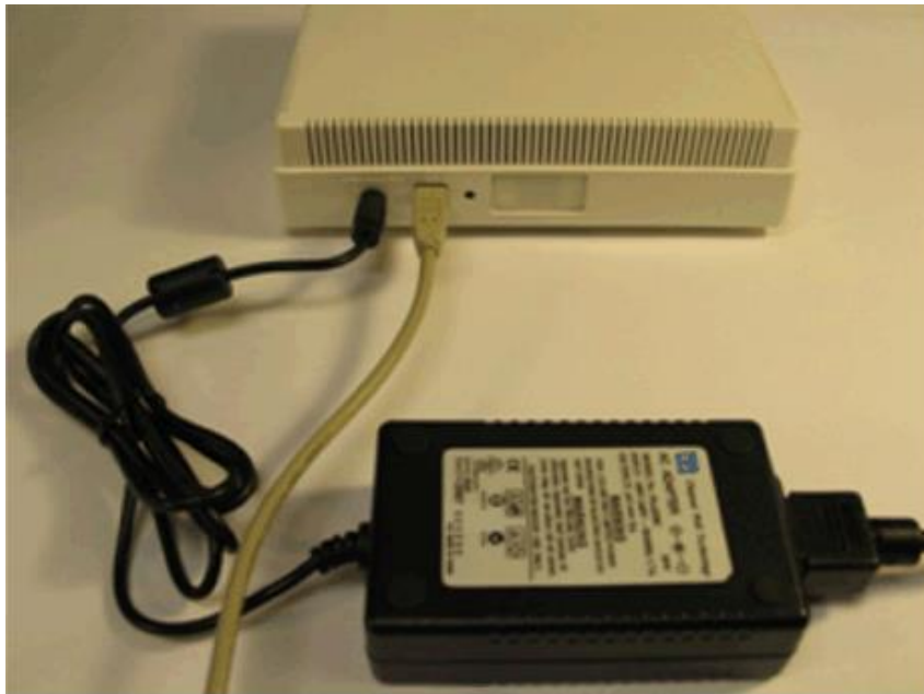
Figure 5 Back view: Power connector and USB connector
